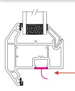
Fit a Sash Spring to the sash on the center line of the stay fixing area
